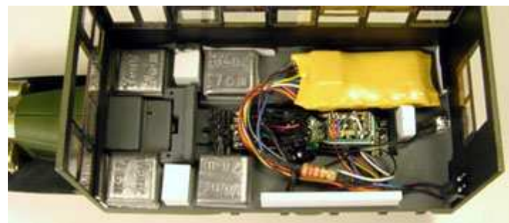
Photo shows placement of Soundtraxx decoder and added weights. We re-used the Bachmann plug to maintain a low profile, but you can raise the mailbox cover with styrene shims to clear a standard NMRA plug.
