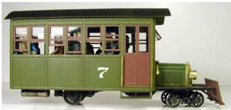
This model was customized with windows raised open to various positions using the "tricky" method described in the instructions. Fuel tank was lowered with styrene shims.
