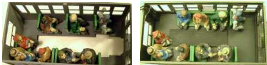
Left: Unmodified figures and kit seats will fit around the Bachmann decoder. Right: Modified figures and false floor used to hide sound components.
