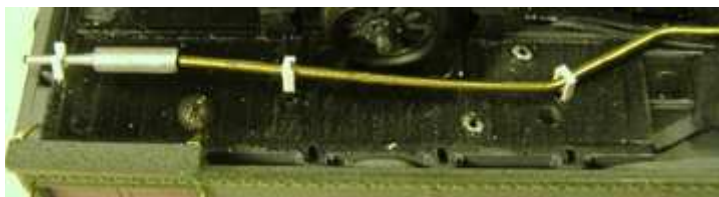
We extended the exhaust on #7 using 3/32" brass rod and hangers made from .080" styrene channel drilled to accept the rod.
